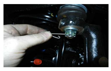
Remove the axle nut keeper and then remove the axle nut.
