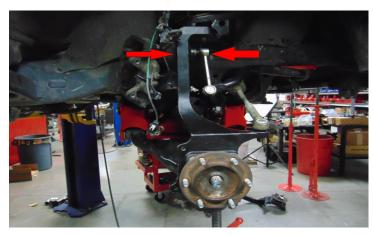
Rotate the tie rod end 180 degree, and attach to the ReadyLIFT steering knuckles. Torque to 60 ft-lbs, then tighten until the castle nut aligns with the cotter pin hole, install cotter pin.
