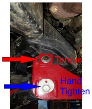
Tighten and torque the passenger differential bolts 75 ft-lbs. Tighten and torque the passenger
