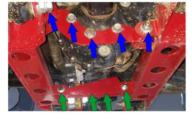
Use a 5/16 or one size larger drill bit to drill out the OEM rear crossmember use the ReadyLIFT crossmember as a guide. Install the nut plate, and fasten the two crossmembers together. Use provided hardware torque to 65 ft-lbs.
