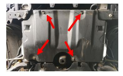
Remove the differential gravel guard.
