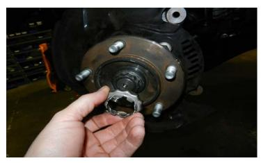
Take care not to damage the threads on the axle. Use an air hammer with a pointed bit in the axle center hole. Slowly press the axle through the hub.
