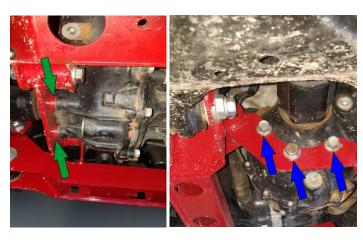
Align the driver side rear differential bracket to the rear crossmember mount, use provided hardware. Do not tighten at this time.
