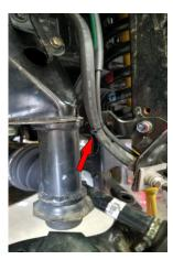
Reinstall the front gravel guard in it's original mounting location. Use factory hardware torque 15 ft-lbs.
