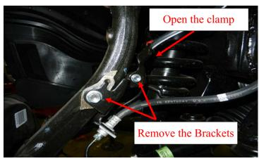
Remove the wheel speed sensor from the steering knuckle.
