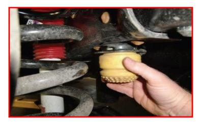
Install the ReadyLIFT bump stop spacer and factory bump stop mount to the frame using M8 x 70 mm bolt and washer. Torque to 5 ft-lbs. Install the bump stop to the factory mount by pressing it back into place.
