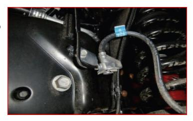
2011 - 2016 front brake line: Loosen the metal line ferrule nut at the rubber brake line block. Rotate the fitting down 180 degrees from factory and tighten. Remove the bracket from the frame.
