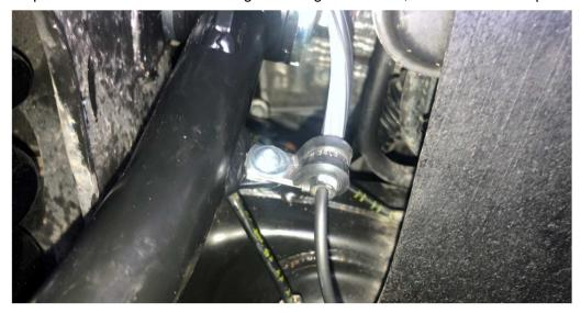
R. At this point, cycle the UCA through its range of motion to verify ABS line clearance and confirm line has enough slack. If there is any contact or not enough slack, adjust position as needed.
