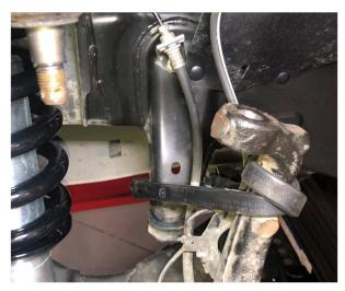
G. Using two 22mm wrenches, remove the nut and washer securing the UCA bolt.
