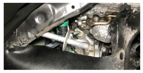
I. For passenger side only, remove the coolant hose clips from the inner fender using a flat head screw driver to allow clearance for UCA bolt removal (the 2 images below are of the right (passenger) side).
