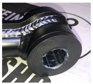
M. Press the steel sleeves into the bushings and apply more grease to outside faces of all bushings and sleeves.
