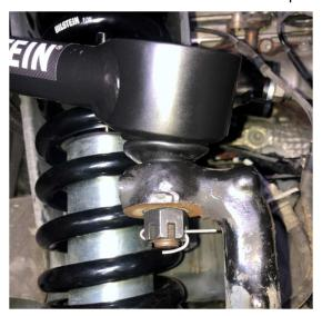
T. Using a 22mm socket and 22mm wrench, torque UCA bolt and flanged nut to 235 Nm (173 ft. lbs.).
