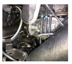
E. Remove cotter pin from upper ball joint castle nut. Using a 19mm wrench, loosen upper ball joint castle nut until flush with the end of the stud.
